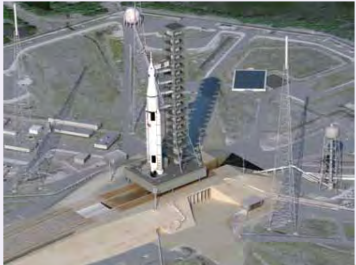
SLS sits on the launch pad in this artist's concept. The launch vehicle will be able to carry the Orion Multi-Purpose Crew Vehicle, as well as cargo and equipment to Earth orbit and beyond. (Credit: NASA)
