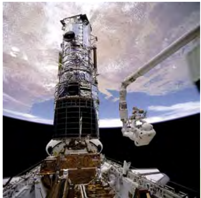
Astronaut Story Musgrave, anchored on Space Shuttle Endeavour's robotic arm, prepares to be elevated to the top of the Hubble Space Telescope during Hubble's first servicing mission, in 1993. Astronaut Jeffrey Hoffman, inside the Shuttle payload bay, assists Musgrave. The mission replaced and repaired various instruments, but its most important task was installing technology that corrected the tiny flaw in Hubble's main mirror that distorted the telescope's view. (Credit: NASA)
