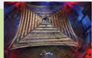
A four quadrant, 65-foot (20-meter) solar sail system is fully deployed for testing in 2005. The design was another solar sail tested by L'Garde, Inc., the company that will be conducting the solar sail demonstration mission for TDM. (Credit: NASA)
