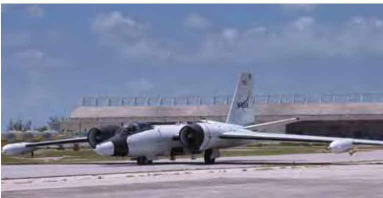
NASA's WB-57 taxis along the runway before going on a MACPEX flight. The wings carry instruments contained in "spearpods" and several other instruments bristle near the underside of the aircraft's nose. (Credit: NASA)
