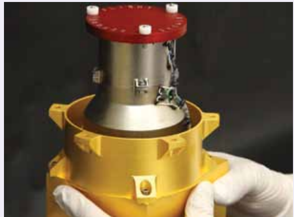
RAD, shown prior to its installation, will monitor high-energy atomic and subatomic particles from the Sun, distant supernovae, and other natural sources. These particles are natural radiation that could be harmful to astronauts on a Mars mission. This image shows the flight hardware with a red "remove before flight" cover on top of the instrument's telescope. (Credit: NASA/JPL-Caltech/SwRI)
