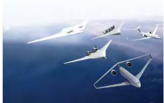
This graphic shows conceptual aircraft designs developed in the Advanced Vehicle Concepts studies. The purpose of the studies was to analyze potential configurations and technologies designed to simultaneously reduce noise, emissions and fuel burn. (Credit: NASA)
