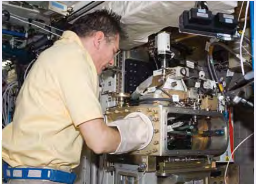
European Space Agency astronaut Paolo Nespoli, Expedition 27 flight engineer, works with the Light Microscopy Module (LMM) in the Destiny laboratory on April 21, 2011. LMM is designed to research colloidal structures, a mixture in which one substance is divided into minute particles (called colloidal particles) and dispersed throughout a second substance. (Credit: NASA)
