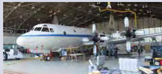
An aerospace engineering student at CReSIS (top) had the opportunity to see the development progress for the fuselage-mounted Multichannel Coherent Radar Depth Sounder (MCoRDS) instrument from a computer aided structural design to the actual installation on the aircraft. The photo below shows MCoRDS being installed at NASA’s Wallops Flight Facility. (Credit, top: CReSIS; below: NASA)
