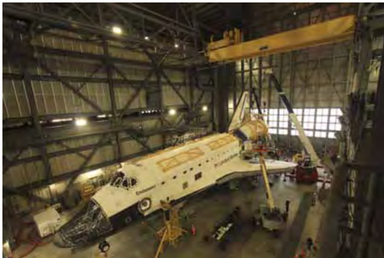
In the Vehicle Assembly Building at NASA’s Kennedy Space Center in Florida, workers lower the cage containing an Approach and Landing Test Assembly (ALTA) pod over the rear of Space Shuttle Endeavour . The ALTA pod is being attached to the site once housing the orbital maneuvering system (OMS) pod. NASA is conducting the demonstration test to ensure the Center’s equipment will fit into the hangar at the National Air and Space Museum when installing an ALTA pod on Shuttle Enterprise . The pod must be reinstalled on a Shuttle for transport on a 747 carrier aircraft. The simulation also tests procedures and timelines necessary to carry out the process. The work is part of the Space Shuttle Program’s transition and retirement processing. (Credit: NASA/J. Grossmann)
